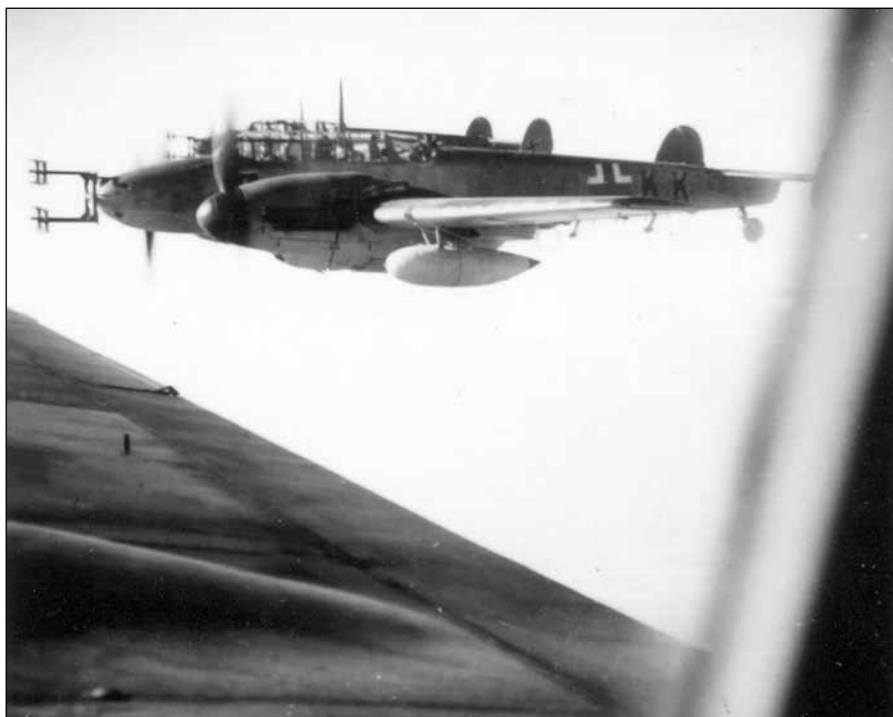
Formation flight of Lichtenstein-equipped Bf110 F-4s of I./NJG4, probably taken in mid 1943. 3C+KK is flying closest to the camera (Coll. Paul Gärtig).
