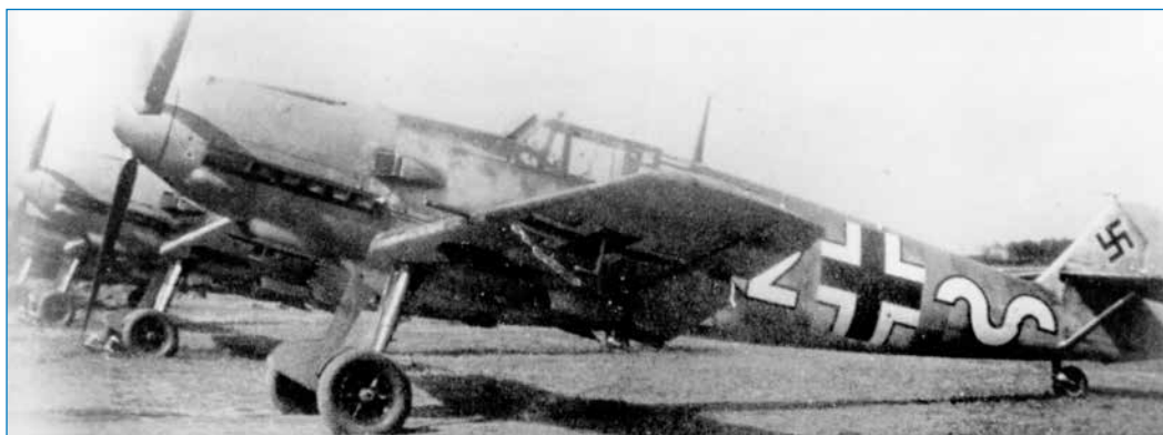
Above: Bf 109E-3, White 12 of 7/JG 52 at Bucharest-Pipera, spring 1941. The Battle of Britain appearance was changed with the yellow engine cowlings, rudders and a narrow fuselage bands behind the fuselage cross. A new feature is the armoured glass on the windscreen.
