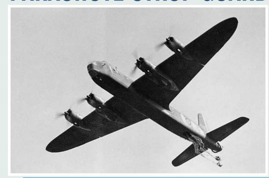
Above: This unidentified Stirling Mk IV, 'O', has its Joe hole open and strop guard lowered, doing the job it was intended for in holding parachute static lines clear of the tailplane. Also visible is the individual code 'O' repeated on the nose, single pitot mast, glider towing bridle and the offset Lorenz rail adjacent to the Joe hole.
