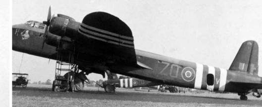
Above: No 295 Squadron's LJ951, 8E-C, shows yet another variation, with smaller, flattened bold letters in the standard Dull Red, with wider spacing between the number and characters. The aircraft carries cut-off invasion stripes beneath the rear fuselage and an indication that those under the wing have been painted out. The rudder and fin also show evidence of repair. LJ951 displays 12 dagger op symbols beneath the pilot's window.
