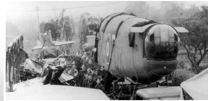
Above: The fuselage of Liberator GR.Mk.III FK221 being removed from Binbrook. QX-C of 224 Squadron crash-landed in bad weather on 19 August 1942. It was later repaired by Scottish Aviation and went to a training unit. FK221 had been delivered on 31 May 1942 and it seems that it retained the original USAAF camouflage. A Boulton Paul Type E tail turret is fitted, note the black turret framing as in Bomber Command aircraft.
