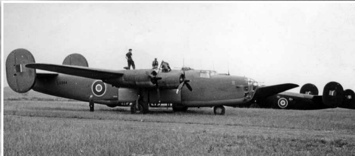
Left: Liberator IIIA LV344 (41-1093) as delivered in standard USAAF camouflage; Dark Olive Drab on upper and side surfaces and Neutral Grey below. In the background are two more RAF Liberators in standard Bomber Command camouflage
