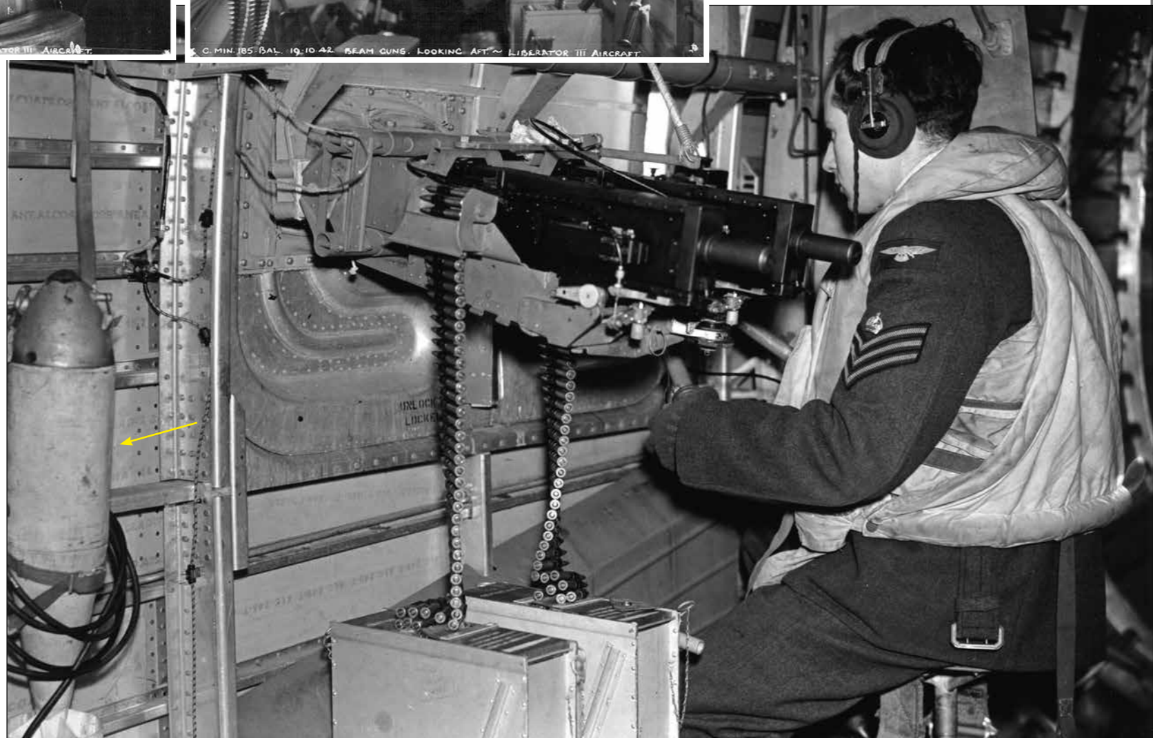
Above right: Beam guns, two pairs of Browning .303 machine guns in FN55 mounts, in a Liberator GR.Mk. III. Armour plates (A) behind the beam positions protect the gunners from attacks from astern.
