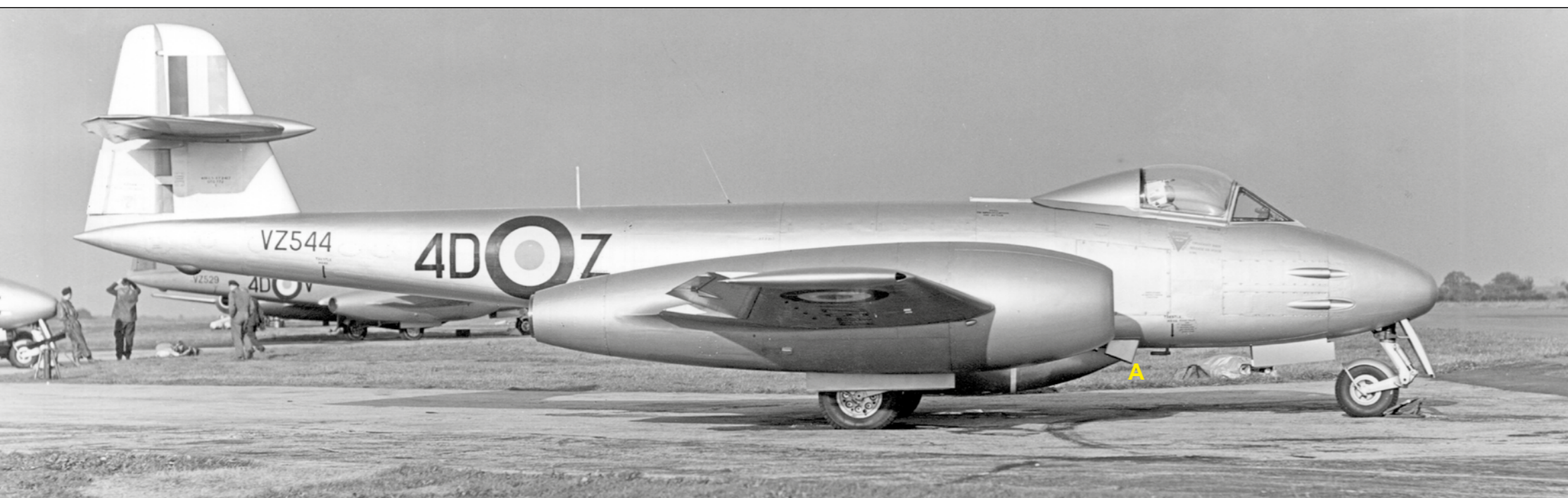
Top: F8s of 74 Squadron including VZ512 4D-D. The lead aircraft shows the marked walkways on the wings. Above: VZ544 4D-Z of 74 Squadron Horsham St Faith, during Exercise Emperor in October 1950. The extended ammunition chutes (A) appear on this aircraft, added as a 'mod' to earlier aircraft. The line slightly forward of this is the 'Trestle Here' marking.
