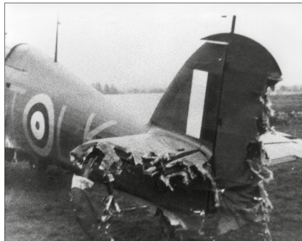
Left: The chewed tail of Johnny Cock's Hurricane after the collision with Trevor Jay's Hurricane. The elevator control must have been marginal to say the least!
