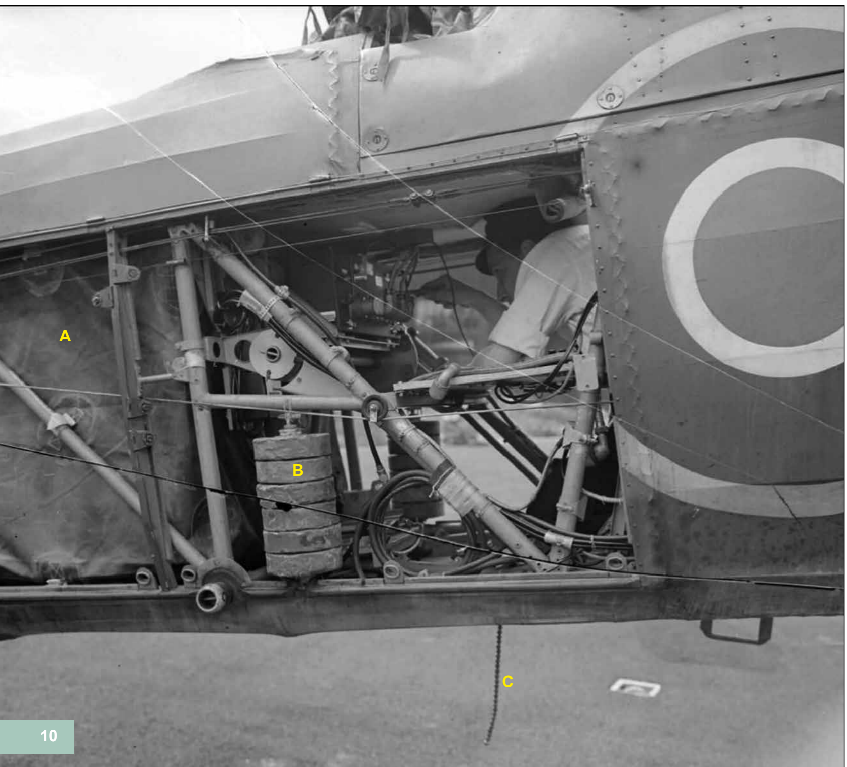
Left: The Swordfish's fuselage interior below the air gunner's position with both side panels removed, showing the type's tubular steel metal framework that was covered in fabric. (A) is a flotation bag, (B) balance weights, (C) lead beads on the end of the trailing aerial. Below: An unusual view of the arrestor hook deployed in flight.
